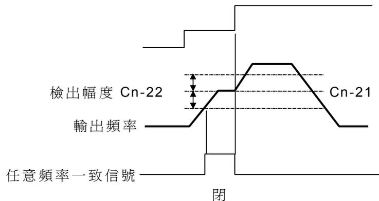
$$(\text{Cn-21} - \text{Cn-22}) \leq \text{輸出頻率} \leq (\text{Cn-21} + \text{Cn-22})$$
