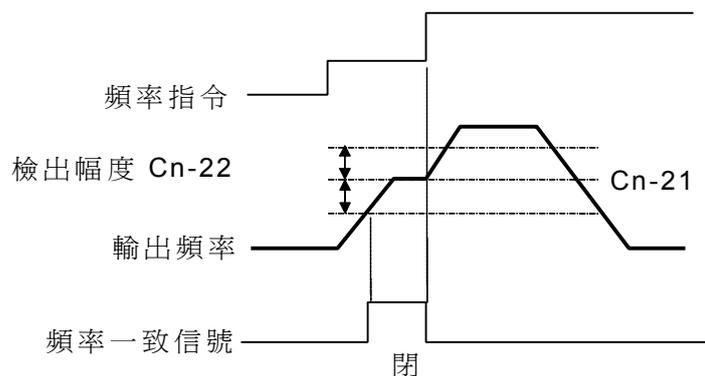
$(\text{Cn-21} - \text{Cn-22}) < \text{輸出頻率} < (\text{Cn-21} + \text{Cn-22})$
